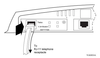
Figure 3-1. Passport 2430 V.34 Modem Adapter Module Connector
